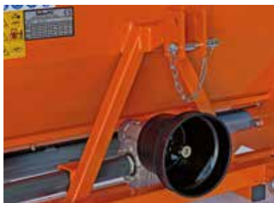
Trasmissione meccanica 540 rpm Mechanical drive 540 rpm Mechanischer Antrieb 540 rpm Transmission mécanique 540 rpm
